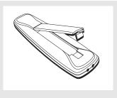
Insert fresh batteries. Make sure that the polarities (+ and -) are aligned correctly.
